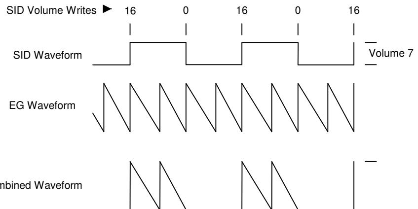
CG EGF SID - Synchronous Sawtooth
